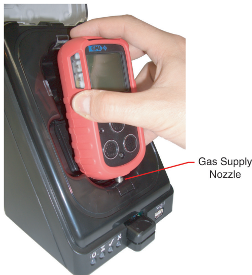
Figure 3-4: Locate Instrument on Gas Supply Nozzle
