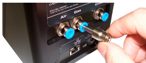
Figure 2-5: Fit 6mm to 1/4 in. Adaptors (if required)
