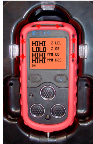
Figure 3-11: Instrument in Alarm Condition
