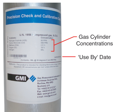
Figure 2-2: Gas Cylinder Label
