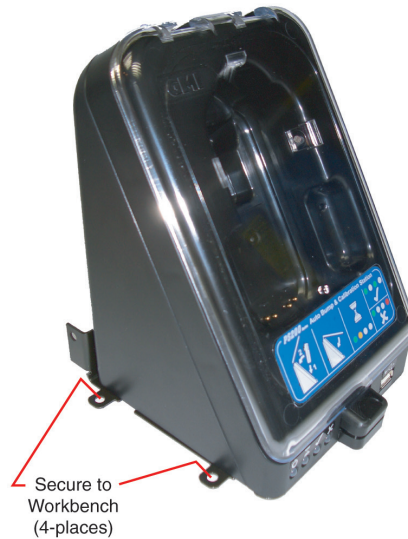
Figure A-3: Attach ABC Station to Workbench
