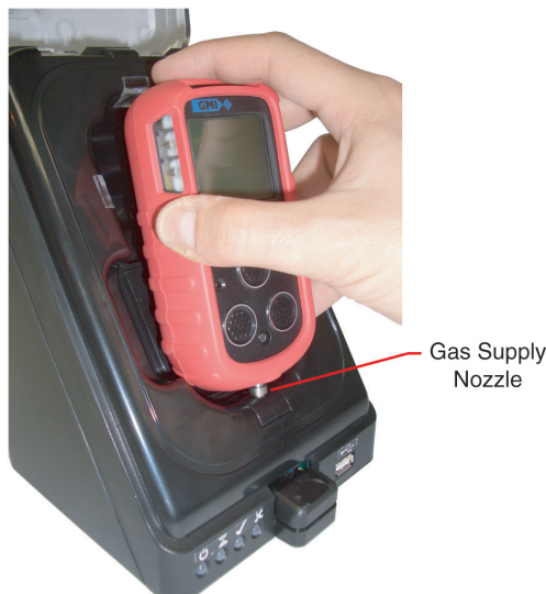
Figure 3-15: Lift Instrument Clear of Gas Nozzle
