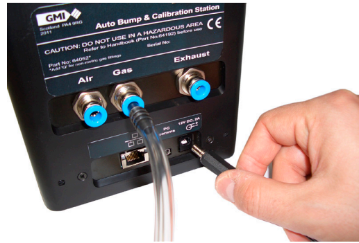
Figure 2-7: Connect Power Supply to Station
