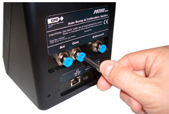
Figure 2-4: Connect Gas Tubing Adaptor to Station
