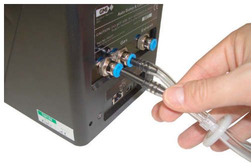
Figure 2-6: Connect Air Tubing Adaptor to Station
