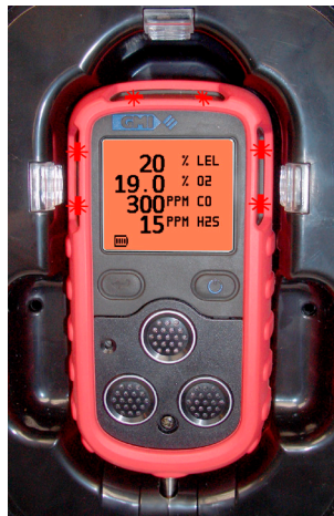
Figure 3-10: Instrument in Alarm Condition
