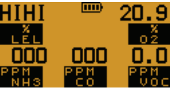
Display in alarm conditions
