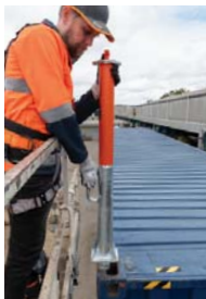
Place container post into ISO corner casting
