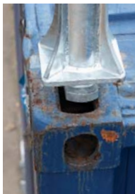
Place container post into ISO corner casting
